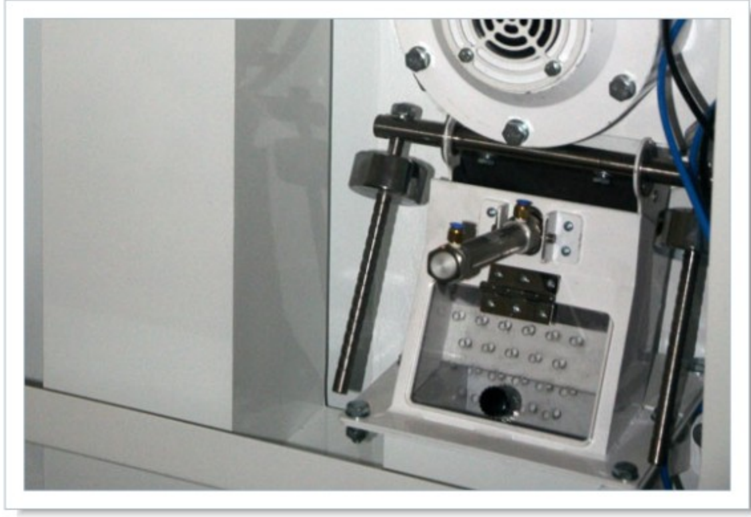
两用压力门 Dual purpose pressure door
